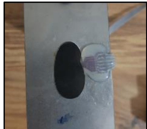
Fig. 7 Strain rosette on shape optimized model
