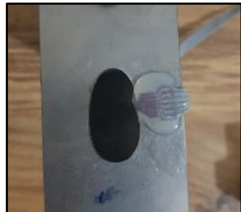
Fig. 7 Strain rosette on shape optimized model
