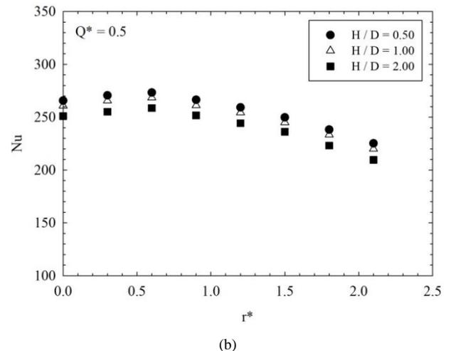
Fig. 4 Variation of the local Nusselt numbers with the dimensionless radial distance as a function of dimensionless nozzle-to-plate distance for different dimensionless flowrate ratio
