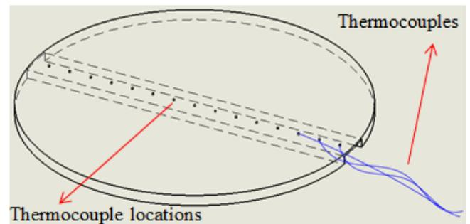
Fig. 3 Detailed view of the copper impingement plate
