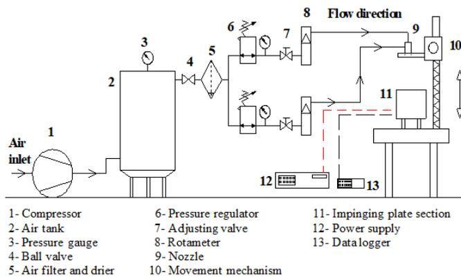
Fig. 1 The schematic diagram of the experimental setup
