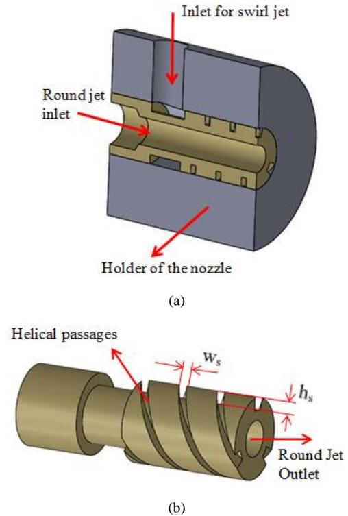
Fig. 2 Solid pictures of the nozzle used in the experiments
