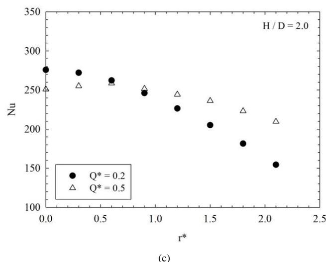
Fig. 5 Variation of the local Nusselt numbers with the dimensionless radial distance as a function of dimensionless flowrate ratio for different nozzle-to-plate distances
