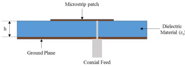
Fig. 1 Microstrip Antenna Structure
