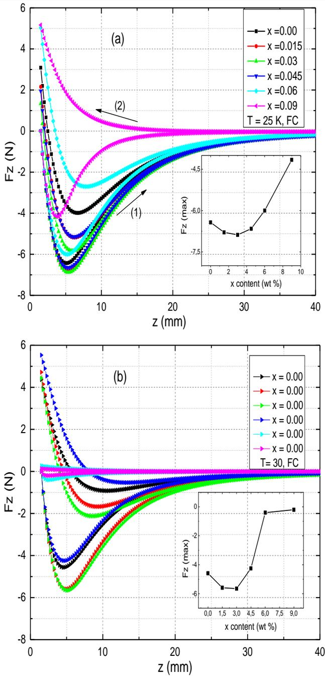
**Figure 3.** The vertical levitation force ( $F_z$ ) versus vertical distance ( $z$ ) for  $MgB_2 + x$  wt %  $C_{22}H_{22}O_6$  bulk samples ( $x = 0, 1.5, 3, 4.5, 6, 9$ ) during descending (row 1) and ascending (row 2) process under FC regime at (a) 25 K (b) 30 K.
