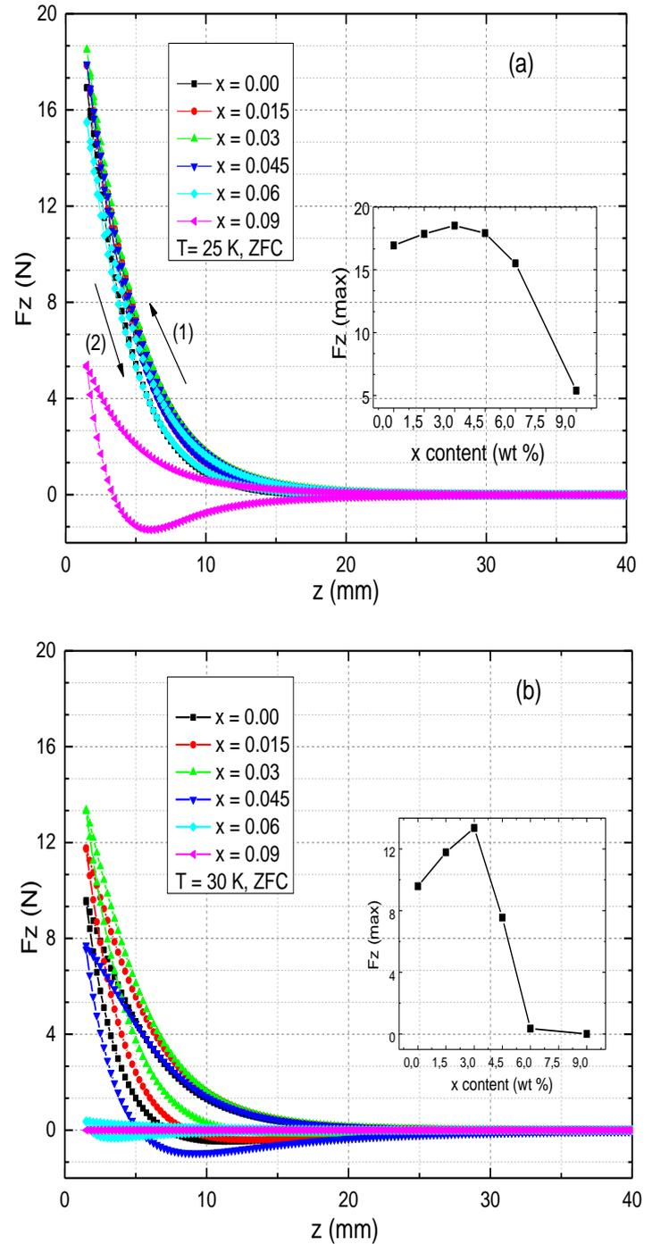
**Figure 2.** The vertical levitation force ( $F_z$ ) versus vertical distance ( $z$ ) for MgB<sub>2</sub>+  $x$  wt % C<sub>22</sub>H<sub>22</sub>O<sub>6</sub> bulk samples ( $x = 0, 1.5, 3, 4.5, 6, 9$ ) during ascending (row 1) and descending (row 2) process under ZFC regime at (a) 25 K (b) 30 K.
