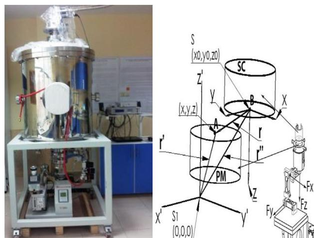
**Figure 1.** The photo and schematic diagrams of magnetic levitation force measurement system.
