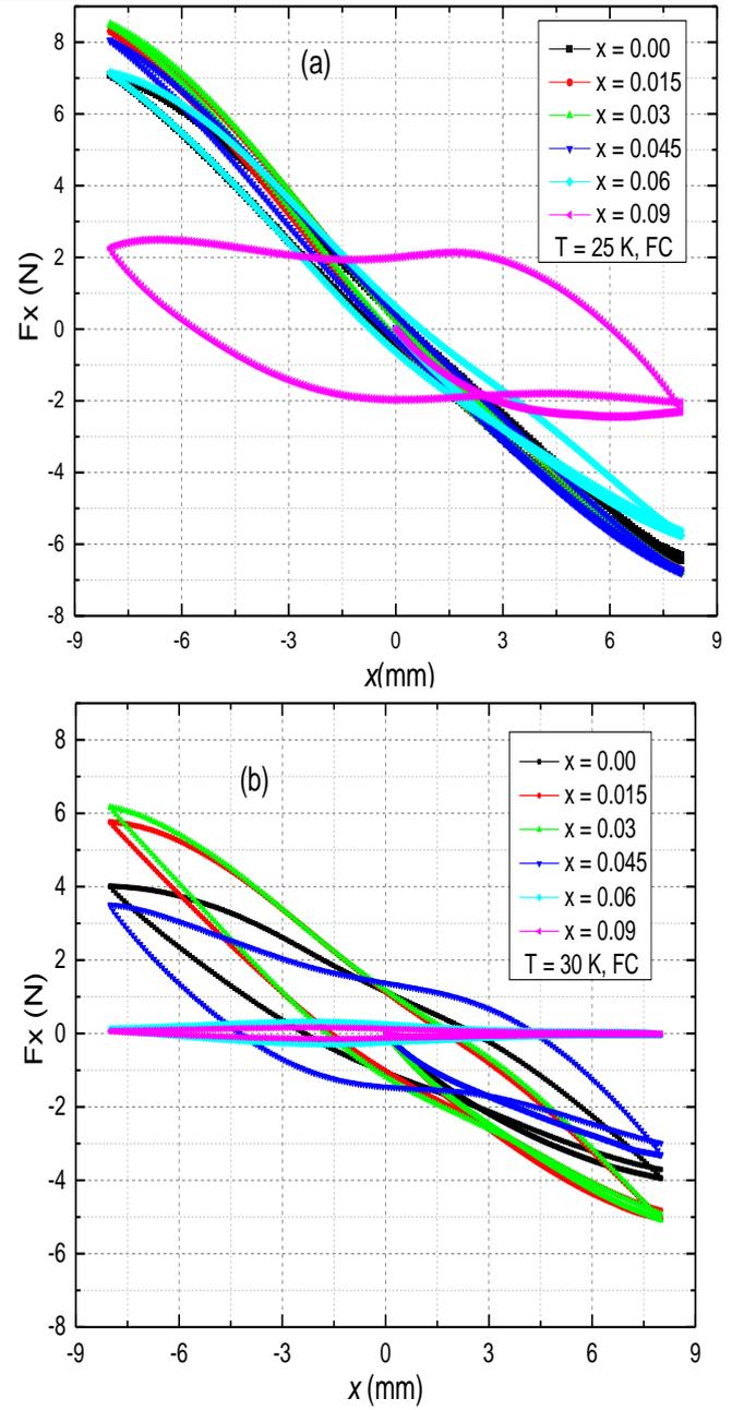
**Figure 4.** Lateral force ( $F_x$ ) versus lateral displacement ( $x$ ) for  $MgB_2 + x$  wt %  $C_{22}H_{22}O_6$  bulk samples ( $x = 0, 1.5, 3, 4.5, 6, 9$ ) under FC regime at (a) 25 K (b) 30 K. The gap between sample and PM was kept 1.5 mm during the test.
