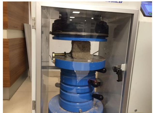
Fig. 7 Compression test of specimens.
