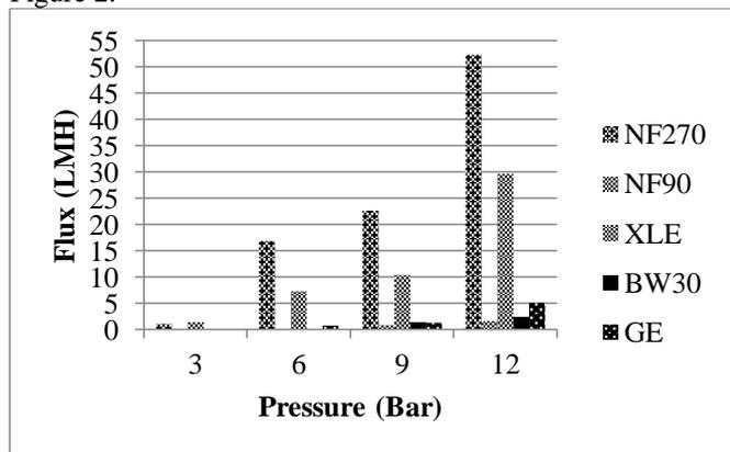
Figure 1. Flux-pressure profile of nanofiltration/reverse osmosis membranes for MF module effluent
