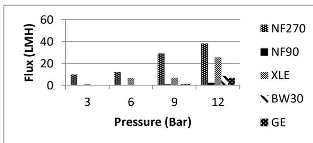
Figure 2. Flux-pressure profile of NF-RO membranes for UF module effluent
