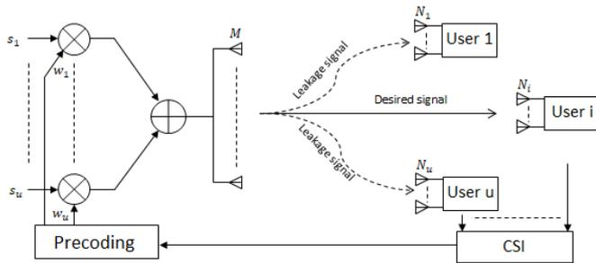
Fig. 1 Block diagram of the MU-MIMO beamforming system use NOMA.
