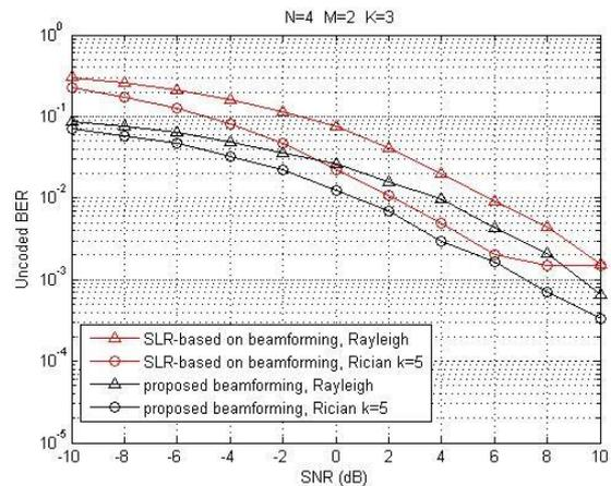
Fig.4 MU-MIMO system for M = 4, U = 3, Ni = 2 over Rayleigh and Rician channel.
