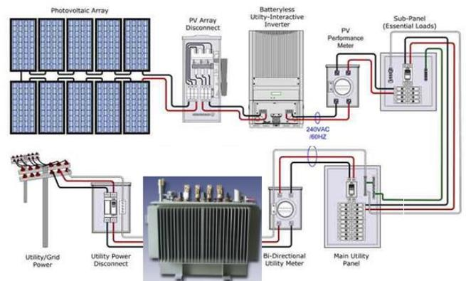
Fig.1b: Block Diagram.
