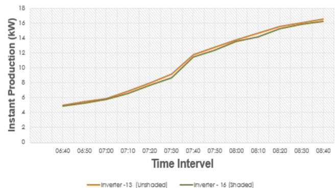
*Fig.3: Instant production for 13 and 16 inverters.*
