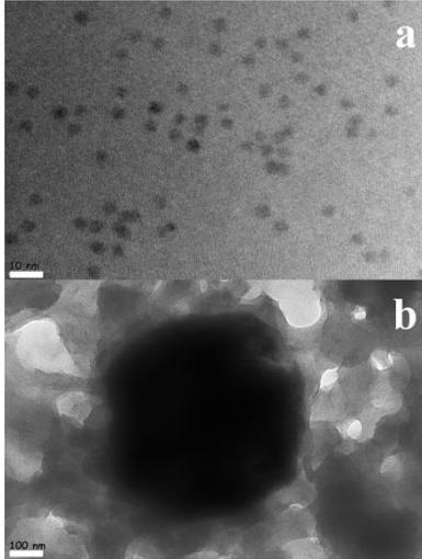
Fig. 2 TEM photos of CdSe nanocrystals and a Bi microparticle. Scale bar is 10 nm for (a) and 100 nm for (b).
