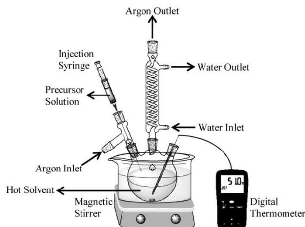
Fig. 1 The synthesis system of the nano- and microparticles.
