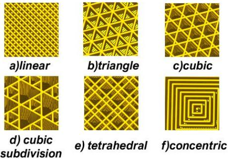
Fig.2 The infill types used in this study.
