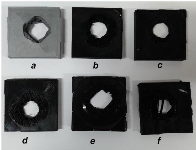
Fig. 5 Tested specimens; a) linear b) triangle c) cubic d) cubic subdivision e) tetrahedral f) concentric
