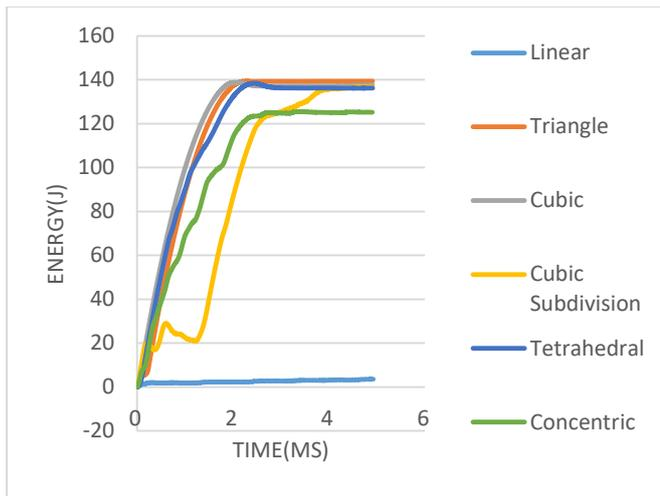
Fig. 3 Effect of infill types
