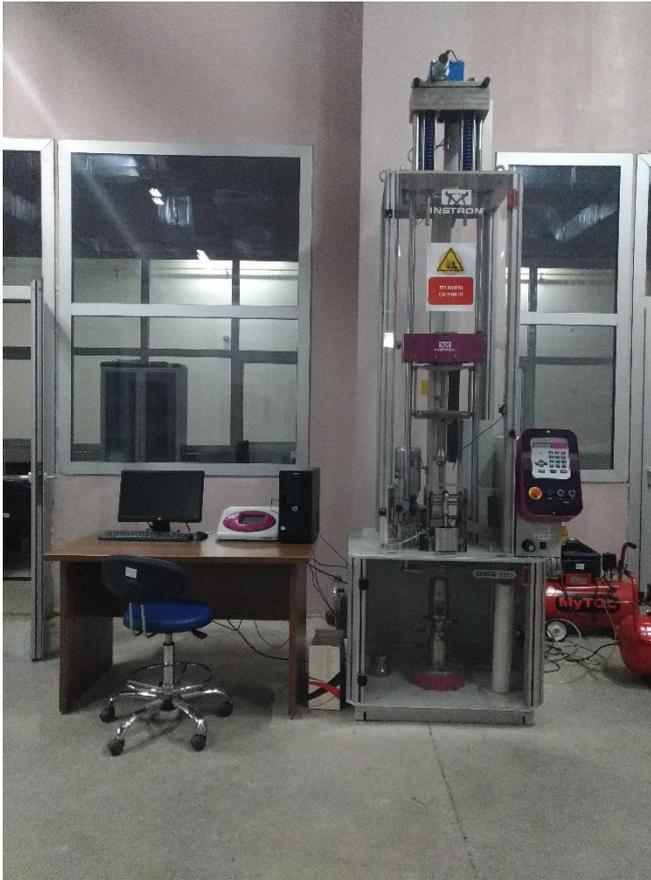
Fig.1 Drop tower impact test system CEAST 9350
