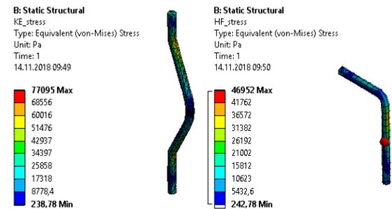
Fig. 15 Equivalent Stress across knee extensor (left) and hip flexor (right)
