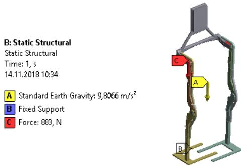
Fig. 11 Constraints and Boundary Conditions
