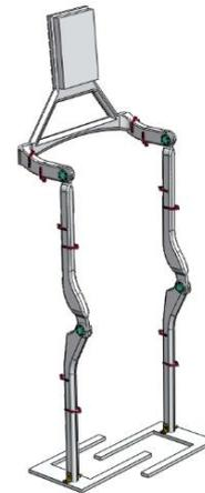
Fig. 2 Pneumatic Muscle Powered Lower Body Exoskeleton
