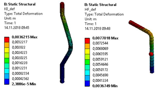
Fig. 14 Total Deformation across knee extensor (left) and hip flexor (right)
