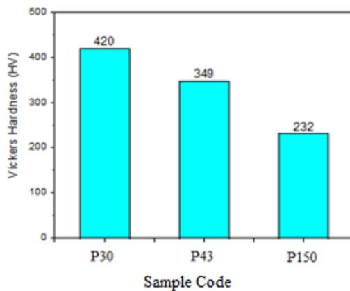
Fig.2. Vickers hardness test results of different powder size of titanium
