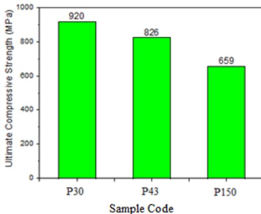
Figure 3. Ultimate Compressive Strength (UCS) test results of titanium powder
