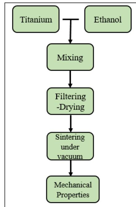
Fig.1.Schematic diagram of titanium fabrication by using PM method
