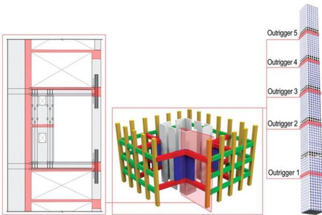
Fig. 3 Outrigger Structural System of 432 Park Avenue
