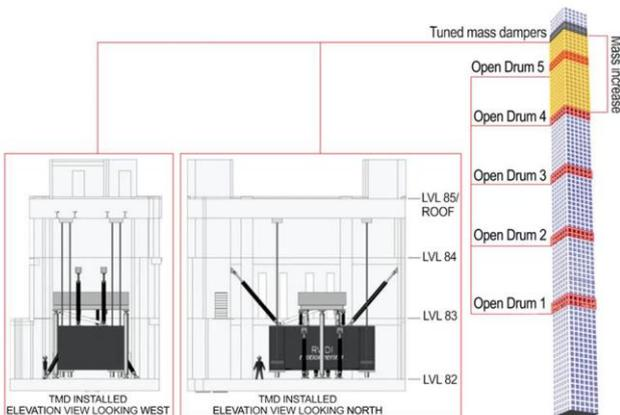
Fig. 4 Open Drum and Tuned Mass Damper Diagram
