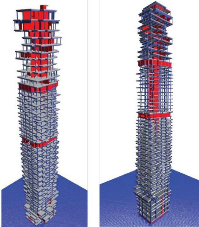
Fig. 9 Diagram for walking columns carrying the loads to shear walls and to the foundation
