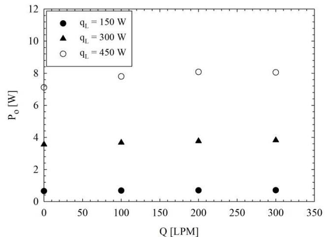
Fig. 4 Effects of both the flowrate and the heat load on the output power
