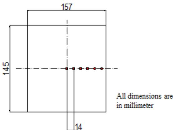
Fig. 2 Thermocouple locations on the back surface of the cell
