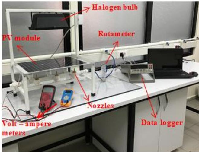
Fig. 1 The photograph of the experimental facility
