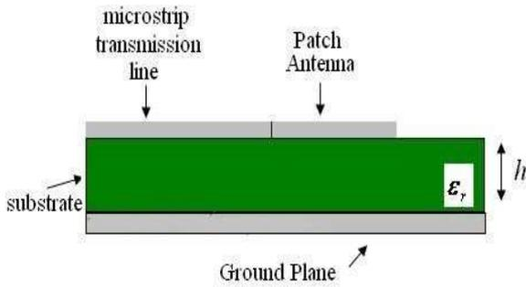
Figure 2. Micro strip patch antenna
