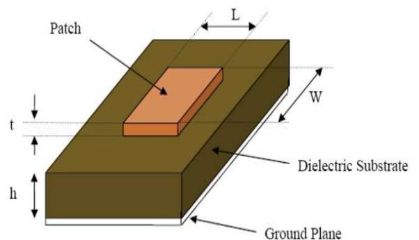
Figure 1: Structure of Micro-strip patch antenna
