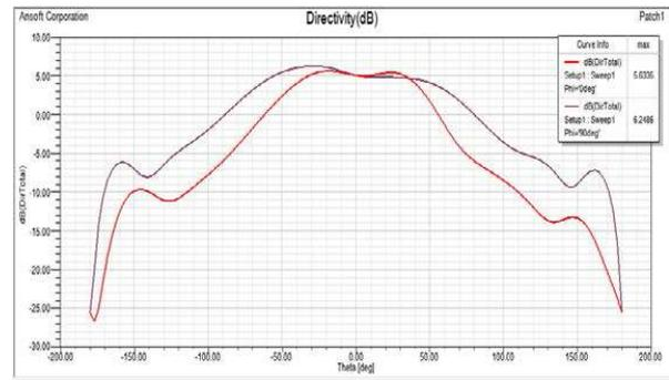
Figure 6: Directivity for Rectangular patch antenna
