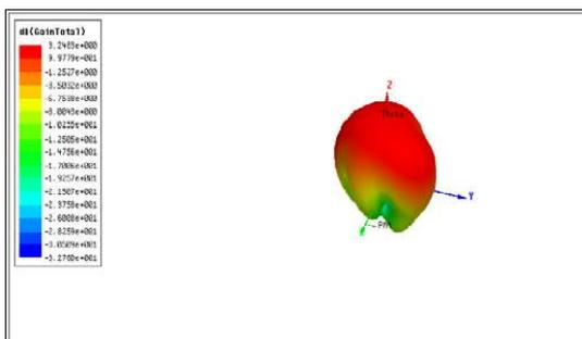
Figure 5: 3d polar plot for Rectangular patch antenna
