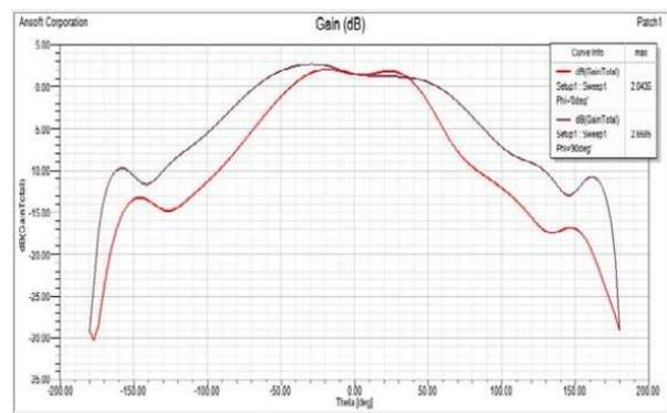
Figure 7: Gain for Rectangular patch antenna
