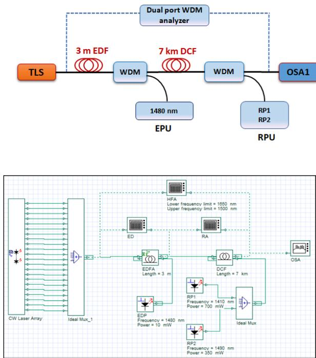
Fig. 1 simulation setup
