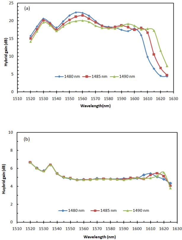
Figure 3. Gain characteristics and NF of S-HFA versus signal wavelength at several RFA pump wavelengths at OPP for signal power of -30 dBm.
