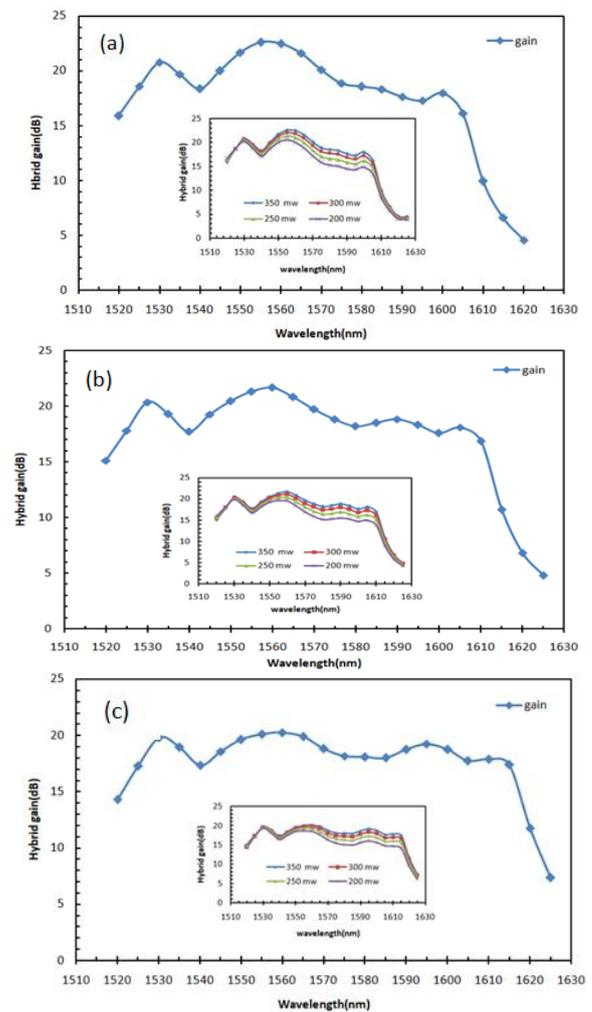
Fig.2 Average gain versus signal wavelength for S-HFA at signal power of  $-30 \text{ dBm}$  and pump power is changed from  $200 \text{ mW}$  to  $350 \text{ mW}$  with a step of  $50 \text{ mW}$ , for the pump wavelength of: (a)  $1480 \text{ nm}$ , (b)  $1485 \text{ nm}$ , (c)  $1490 \text{ nm}$  and.
