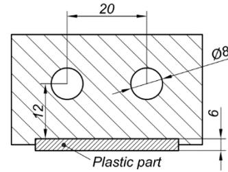
Fig. 2 Section and dimensions of cooling channels
