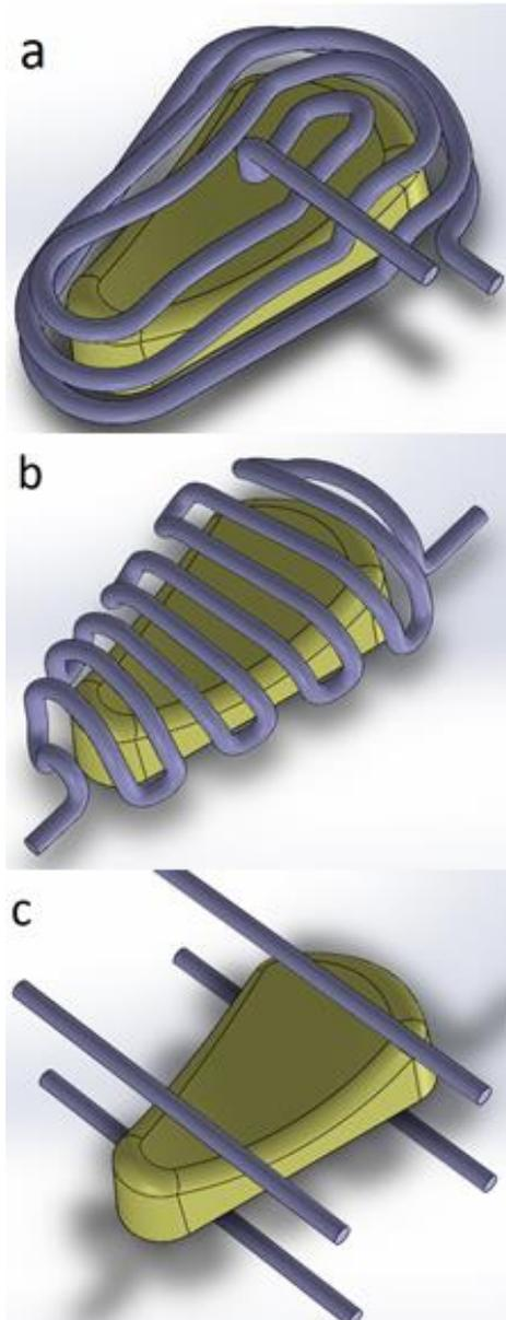
Fig. 4 Spiral, Zig-zag and straight cooling channels
