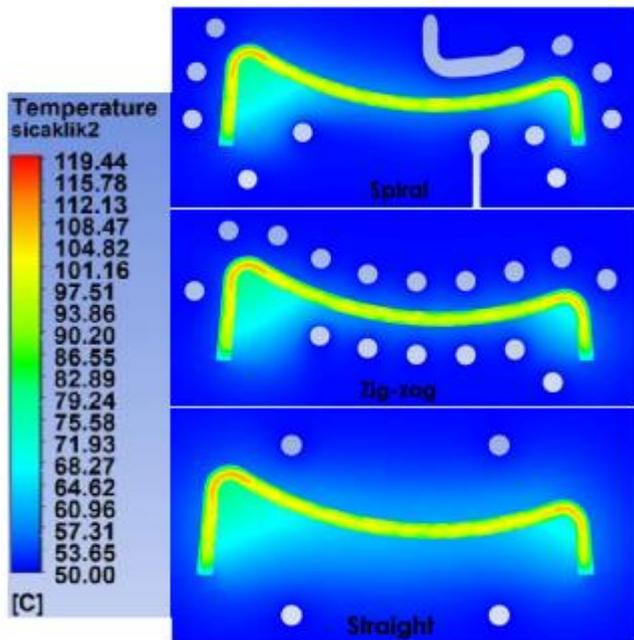
Fig. 6 Temperature distribution on section at 48<sup>th</sup> second of cooling process
