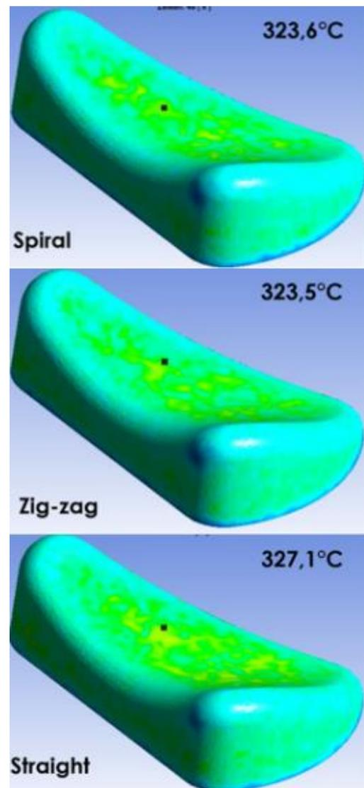
Fig. 5 Temperature distribution on part surface at 48<sup>th</sup> second of cooling process
