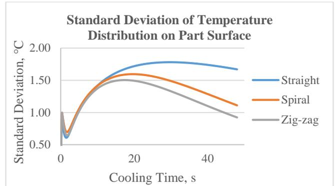
Fig. 8 Standard deviations of temperature distribution on plastic part surface
