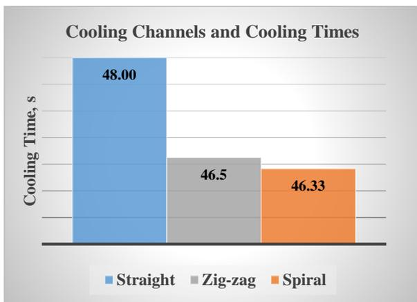
Fig. 7 Cooling times
