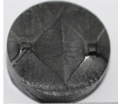
Fig. 1. The photo of two-seeded cylindrical YBCO superconductor fabricated by MSMG method
