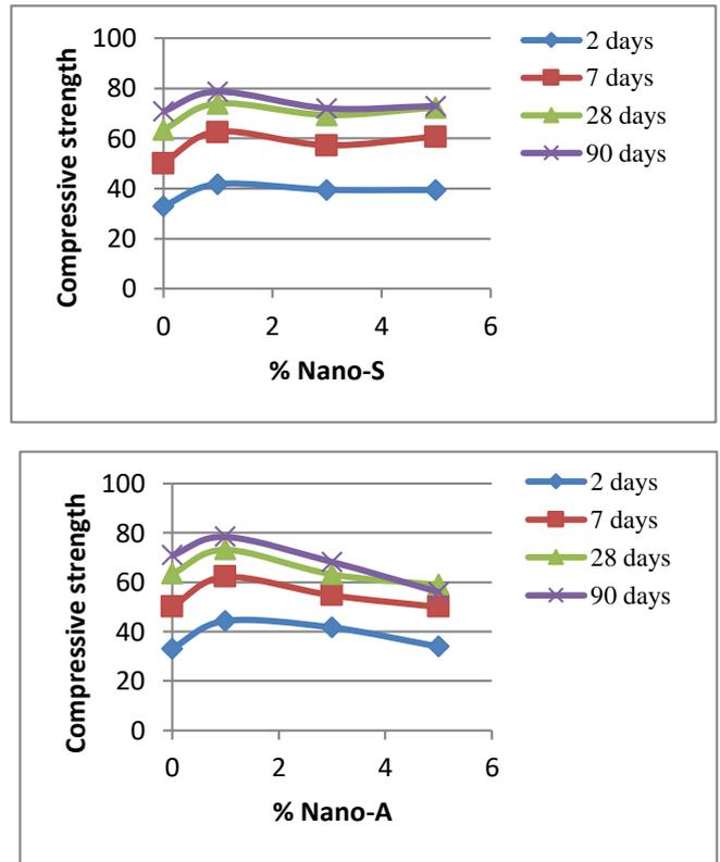
Figure 1.a-b Nano-SiO<sub>2</sub> and Nano-Al<sub>2</sub>O<sub>3</sub> powders additives samples of 2, 7, 28 and 90 days compressive strength results were compared to the reference sample
