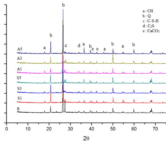
Figure 2. Results of XRD analysis of the specimens with the addition of nano powders in different percentages
