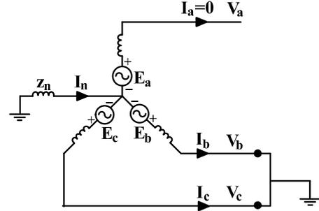
Fig. 3 Double line-to-ground fault in unbalanced-unloaded synchronous generator
