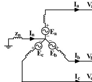
Fig. 1 Circuit diagram of the unbalanced-unloaded synchronous generator where the generator's neutral is grounded through an impedance
