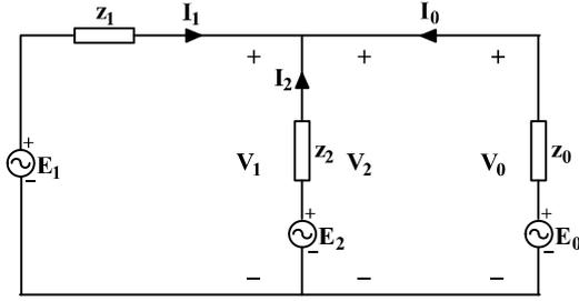
Fig. 4 Equivalent short circuit model for double line-to-ground fault in unbalanced-unloaded synchronous generator
