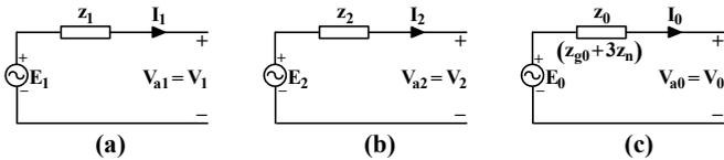
Fig. 2 Unbalanced-unloaded synchronous generator sequence circuit model a) positive sequence circuit b) negative sequence circuit c) zero sequence circuit
