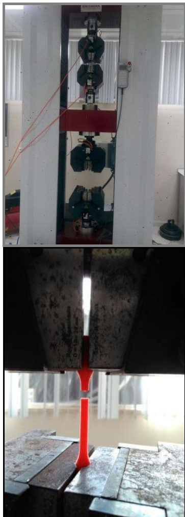
Figure 5 Tensile test machine and damaged sample
