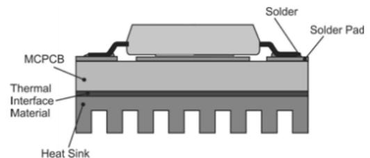
Fig 2. Schematic representation of a LED [4].
