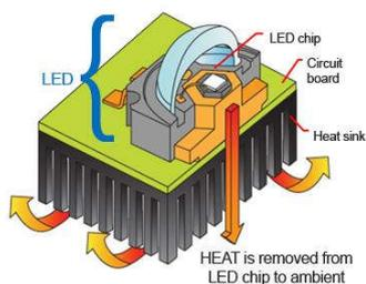
Fig. 2. Schematic representation of heat flow on LED package and thermal management parts [2].
