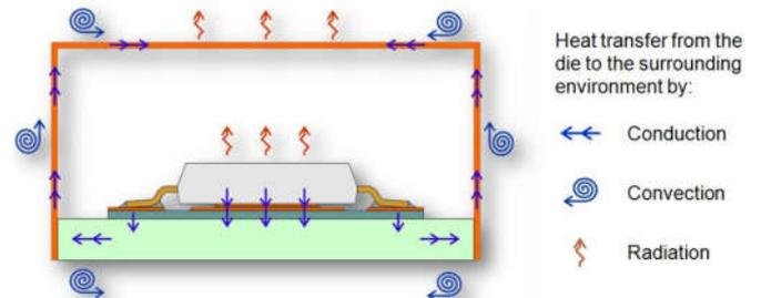
Fig. 3. Heat transfer mechanisms in LED package [3]
