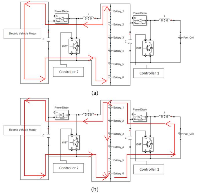
Fig. 5 (a) Battery supplies energy into the motor and (b) Fuel cell both charges the battery and drives the motor
