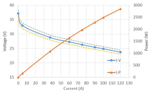
Fig. 3 DuraPEM W240 fuel cell stack steady state I-V and I-P characteristics
