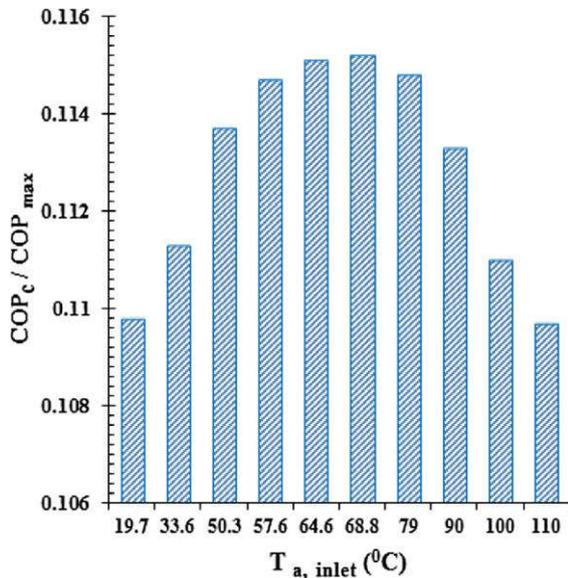
Fig. 18: The effect air inlet temperature on COP<sub>c</sub>/COP<sub>max</sub>. [20]
