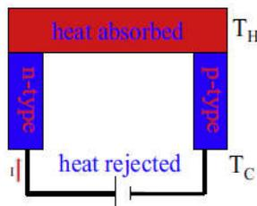
Fig.1: The schematic diagram of thermoelectric cooler.[3]
