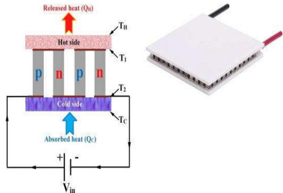
Fig.4: Schematic diagram of a single-stage thermoelectric device.[10]
