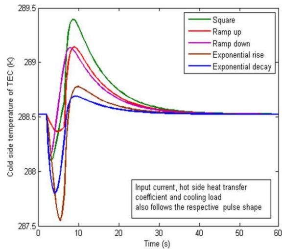
Fig. 12: Cold side temperature of TEC for different pulse shapes [16]
