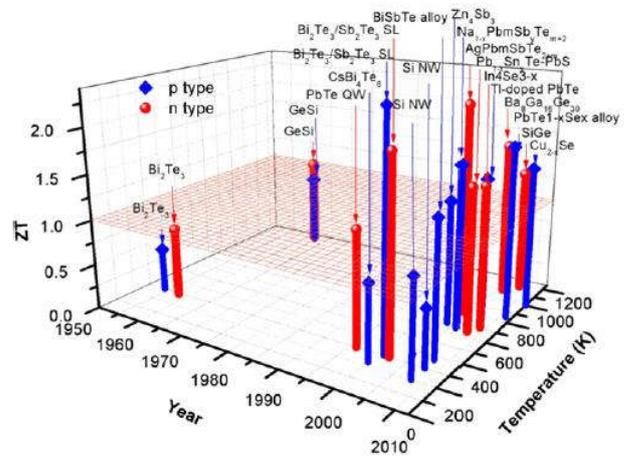
Fig.3: ZT as a function of temperature and year revealing the important development of thermoelectric materials[9].
