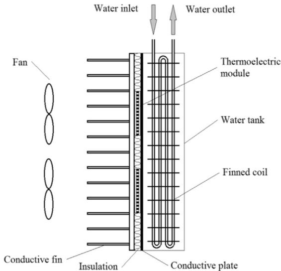
Fig.15: Schematic diagram of the thermoelectric cooling unit[18].
