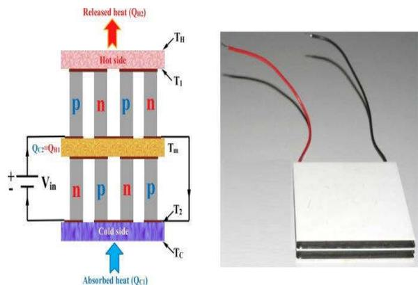
Fig.5: Schematic diagram of a two-stage thermoelectric device[10]
