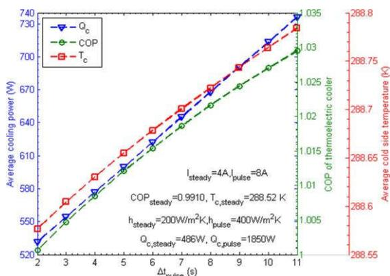
Fig. 11: Variation of average cooling power, COP and average cold side temperature with different pulse width [16].
