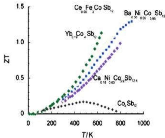
Fig 2: ZT as a function of temperature for skutterudites [9]
