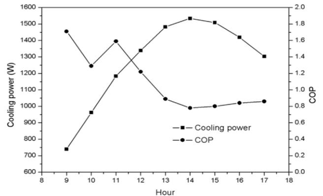
Fig. 16: Thermoelectric system's cooling performance during the cooling period [18].
