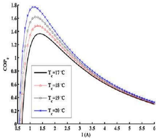
Fig. 10: Relationship between COPc and electrical current [15]
