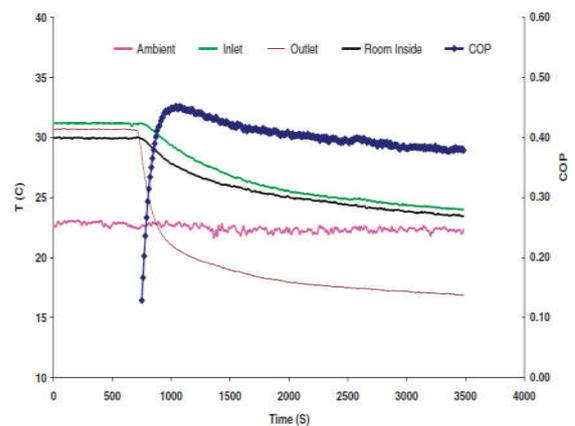
Fig.13: Temperature and COP variations for model room testing [17].
