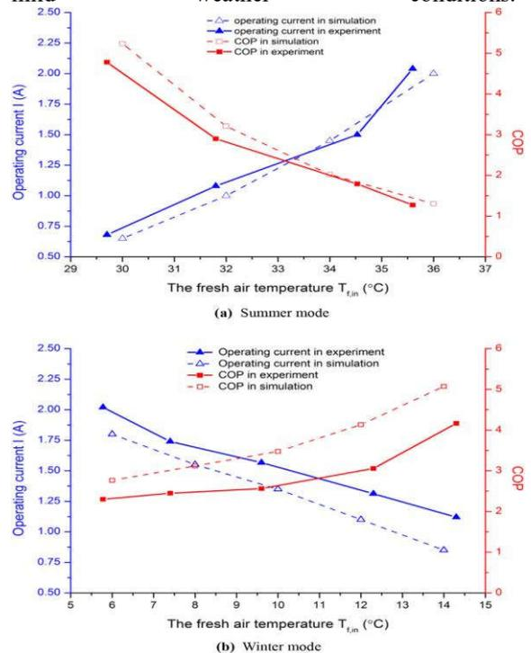
Fig.17: Operating current and COP under different fresh air temperatures[19].
