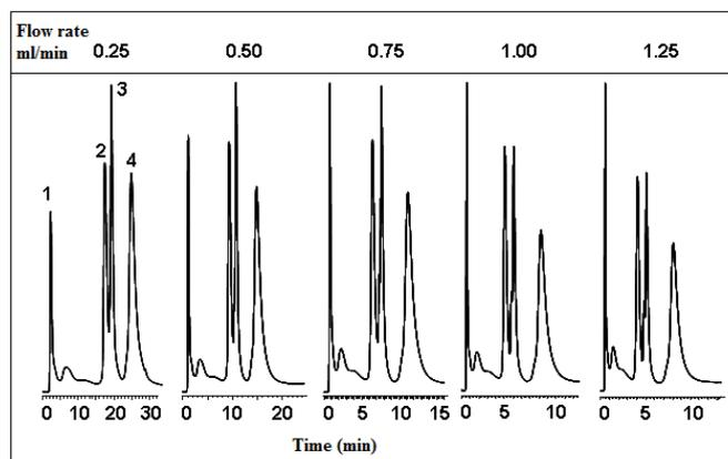
Fig. 3 Sample chromatograms showing protein separation under gradient conditions by ion exchange chromatography using column containing poly (MAA) -grafted poly (DHPM-co-EDM) particles synthesized by AH Mobile phase: A: 20 mM HEPES buffer (pH 8), B: 20 mM HEPES buffer (pH 8) + 1 M NaCl, Gradient conditions: 100% A to 100% B in 20 min. Column dimensions: 50x4.6 mm i.d., UV-detector 280 nm. Peak order: (1) Myoglobin, (2) Ribonuclease A, (3) Cytochrome C, (4) Lysozyme.
