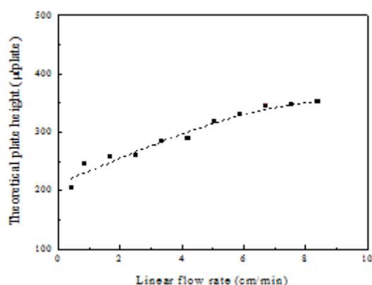
Fig. 4 Alteration of plate height by linear flow rate for columns containing poly (MAA) -grafted poly (DHPM-co-EDM) particles obtained by AH. Analyt: Cytochrom C (0.25 mg / mL), Column dimensions: 50x4.6 mm i.d., UV detector, 280 nm. Mobile phase: pH 8, 20 mM HEPES buffer + 1 M NaCl
