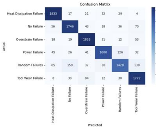
Fig. 7 Confusion Matrix from Random Forest after CTGAN Augmentation. Confusion matrix from Random Forest after CTGAN augmentation, showing correctly classified failure types.
