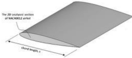
Fig. 1. Figure of the NACA0012 airfoil pitching sinusoidally at a center of the quarter chord point, with amplitude ( \Delta\alpha ) and frequency( f ) around a mean angle of attack( \alpha_m ) in a uniform flow ( U ) and the rotation formula is \omega = \alpha_0 + \alpha_m \sin(2\pi ft)
