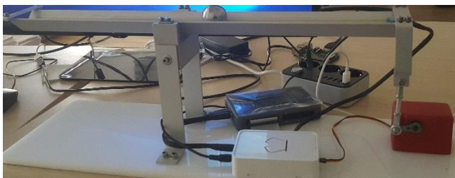
Fig. 2 The Ball and Beam System, Acrome.
